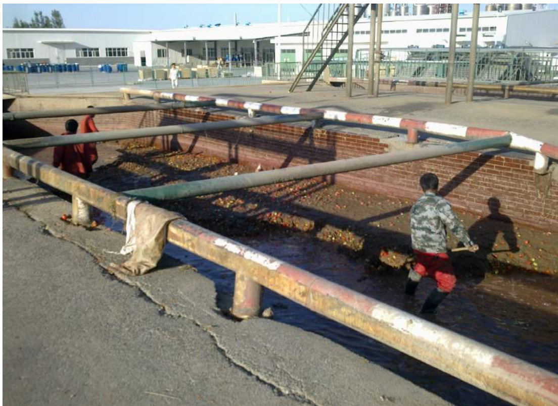
Photo: Waste water generated from the processing step is being separated from solid waste in a processing pool. By SRI
