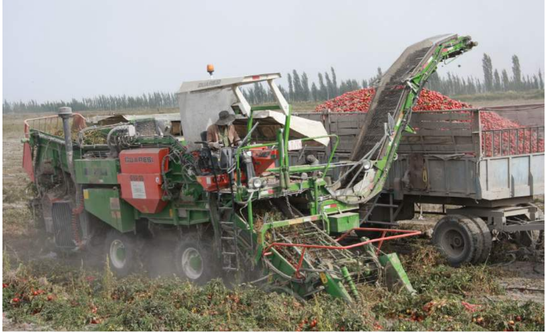
Photo: A plucking machine is working and a transport vehicle is following it to collect tomatoes By SRI
