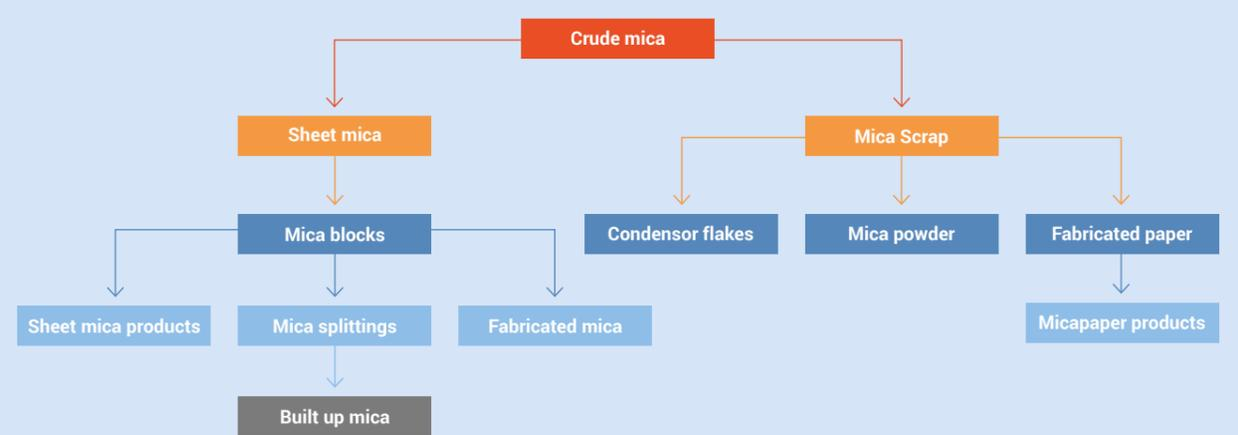
Figure 5: Flowchart of mica production
