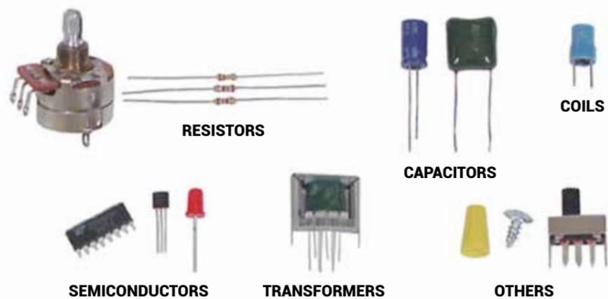
Examples of electronic components mounted on PCBs.<sup>103</sup>
