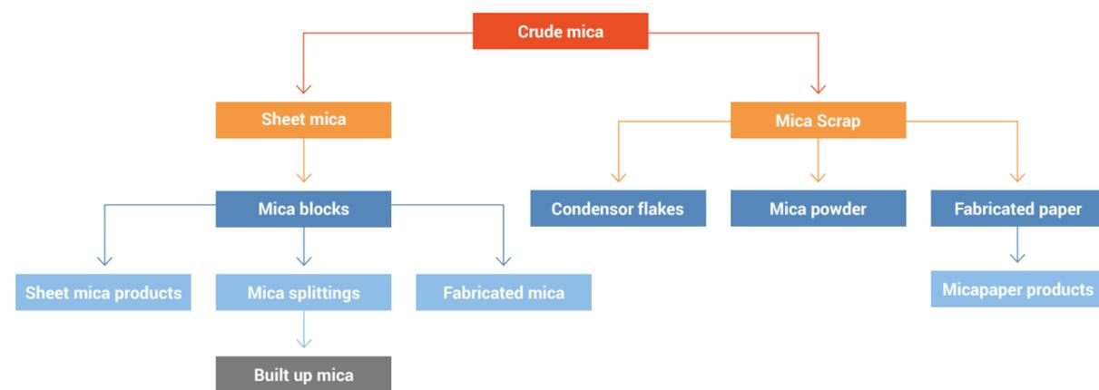
Figure 1: Flowchart of mica production Source: Gunpatroy Pvt. Ltd, adapted by SOMO.
